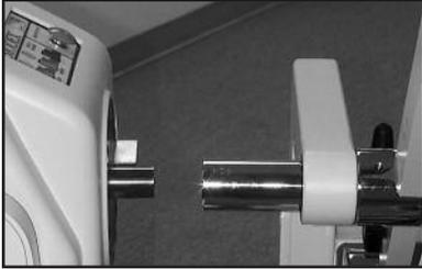
*Figure 5. Align the connecting hub red dot with the dynamometer shaft red dot.*
