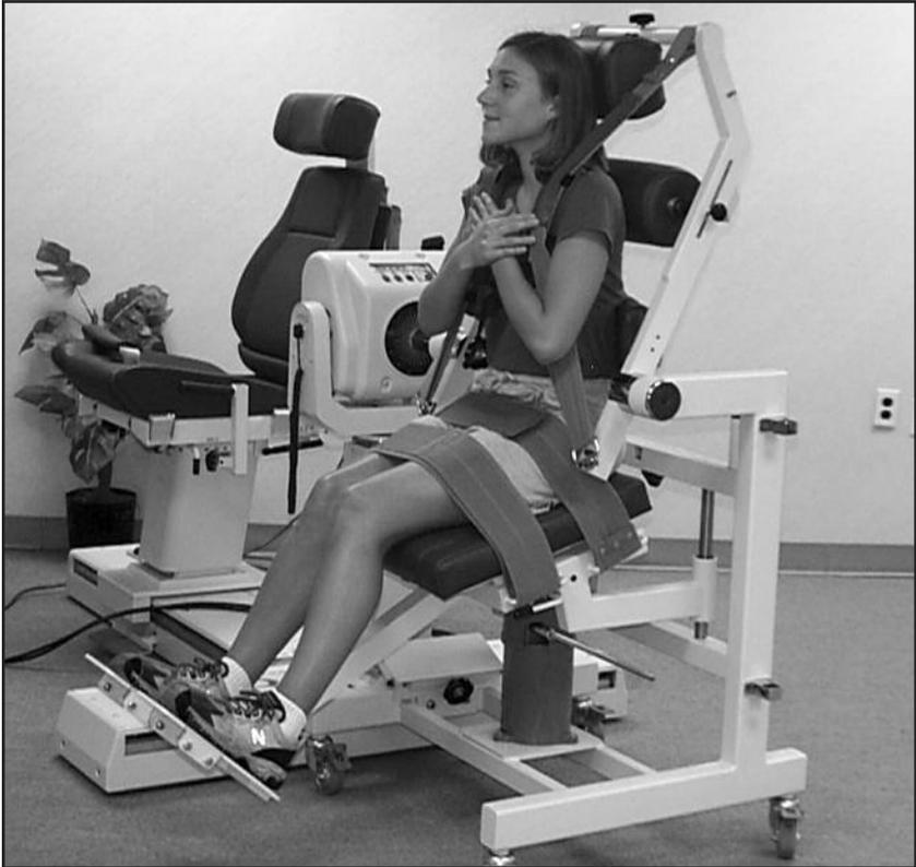
*Figure 1: The Biodex Multi-Joint System with Dual Position Back Ex/Flex Attachment. The patient is exercising in the semi-standing (functional) position. For exercise or testing in the seated-compressed position, remove the lumbar pad, raise the seat to the inclined position, and insert both the sacral pad and lower extremity compression device.*
