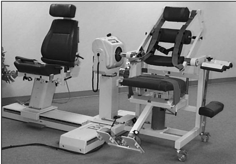
Figure 4. The Biodex Dual Position Back Ex/Flex Attachment secured to the Biodex Multi-Joint System.
