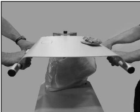
*Figure 3: Using two people, grab the handles on the upper rack to remove unit.*
