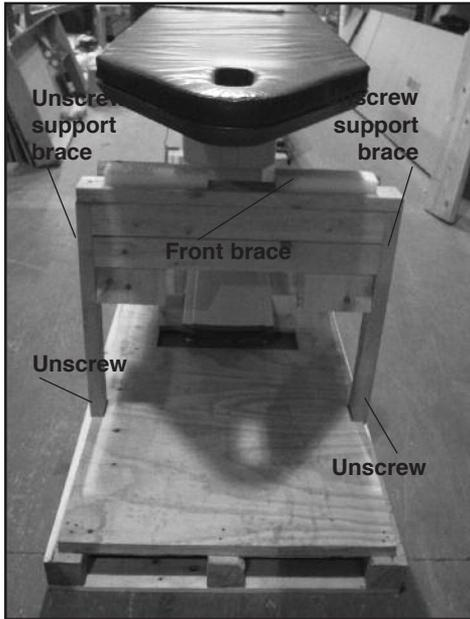
*Figure 1: The front brace is positioned under the front end of the table. Use the Hand-Held Controller to raise the tabletop, then unscrew the brace from the skid and the angled brace supports from the brace. Lift up on the brace to remove it from the shipping crate.*
